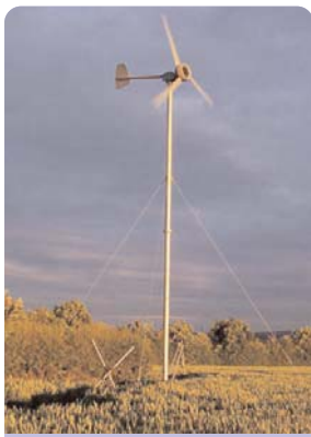
A 5.3kW Iskra wind turbine (Iskra)
